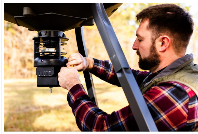
Figure 1: Installing the 6V battery into the feeder kit.
