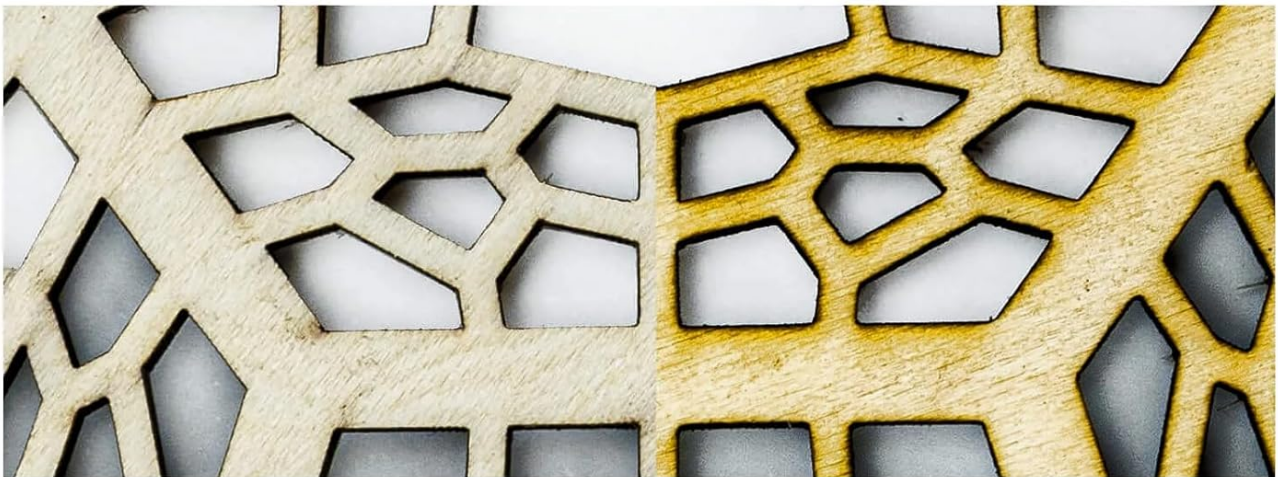
Image: A side-by-side comparison demonstrating the superior cleanliness and quality of laser-cut wood when using the ATOMSTACK F60 Air Assist (left) versus without air assist (right).
