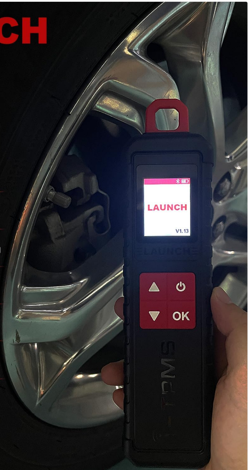
Figure 3: A user holding the i-TPMS tool next to a car tire, demonstrating the activation process. The tool's display shows "LAUNCH" and version information.
