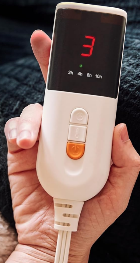
Image 5.1: Digital controller displaying heat and timer settings.
