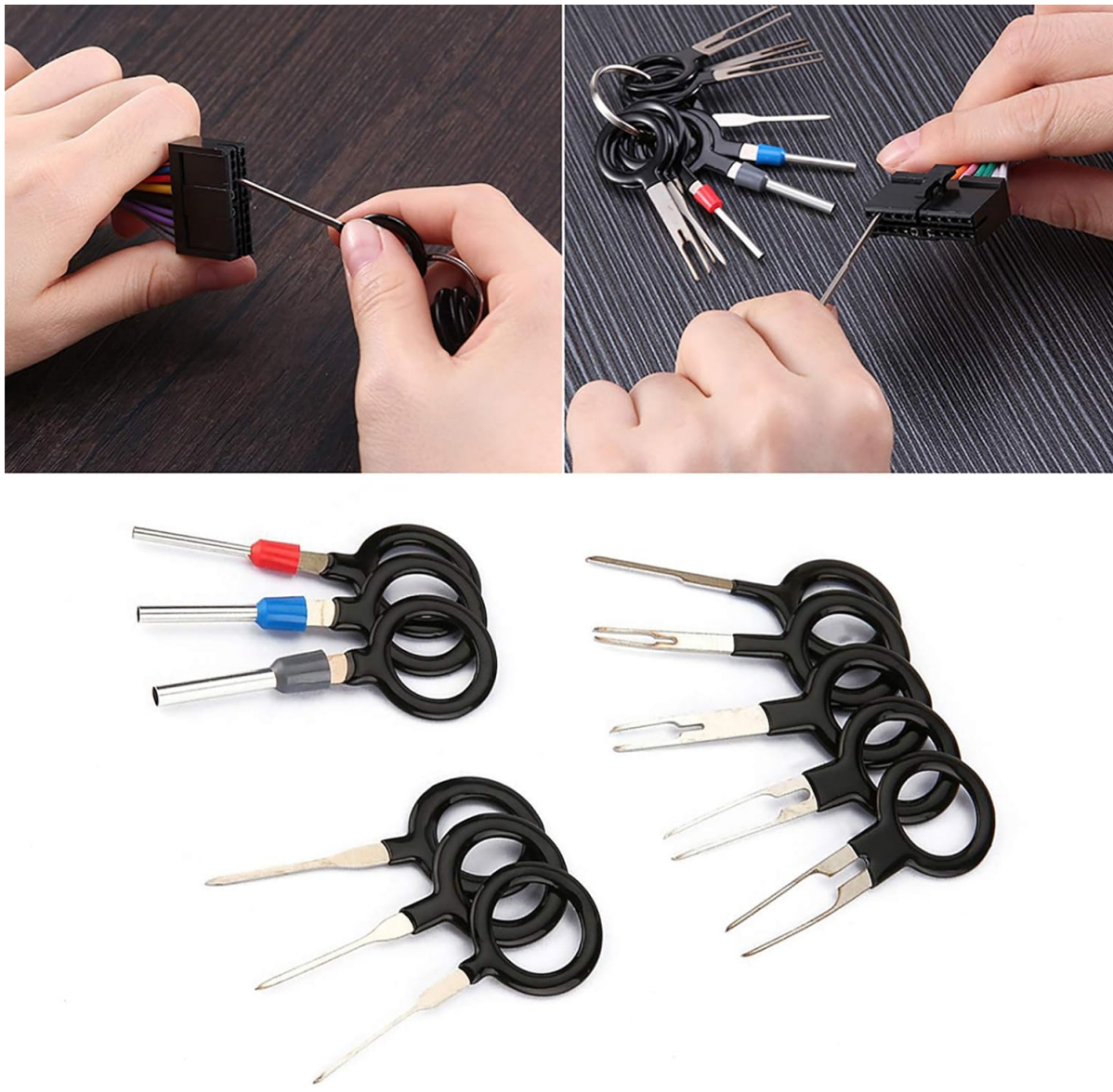
Image 5: A composite image showing various tools from the kit and their application in removing terminals from different types of connectors.
