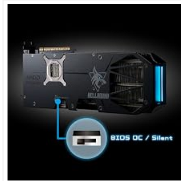
Illustration of the Dual BIOS switch, allowing selection between OC and Silent modes.
