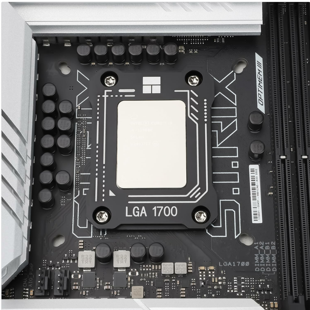
Image 4.3: Top-down view of the retainer installed, showing even pressure distribution.
