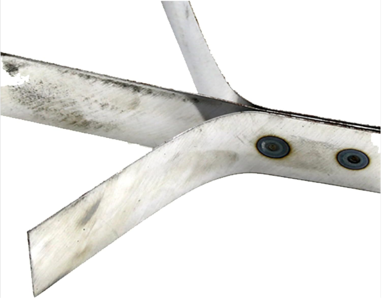
Figure 6.4: Visual representation of a successful spot weld, showing the fused area between two metal pieces.
