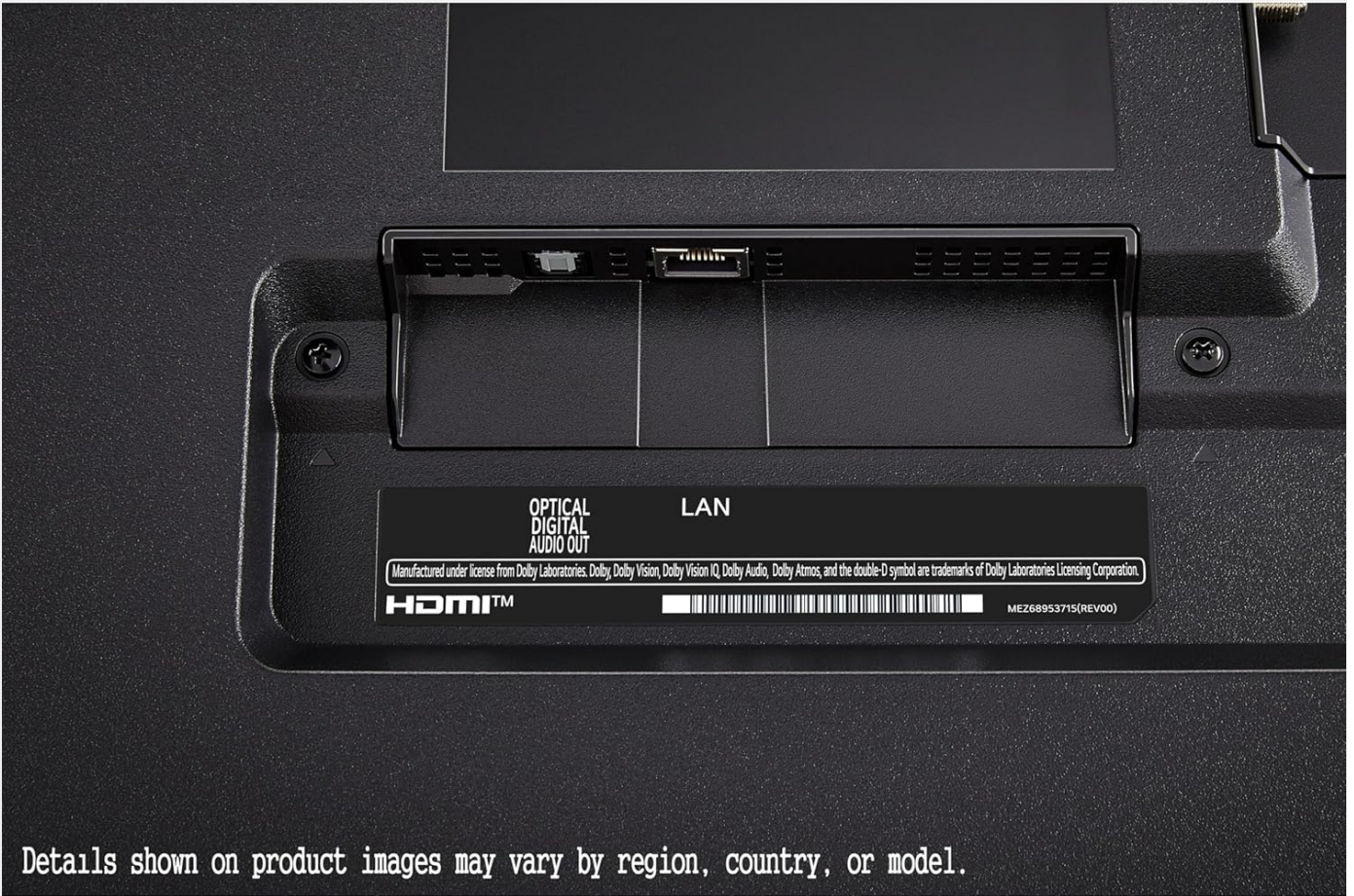
Figure 3.3: Close-up of Optical Digital Audio Out and LAN ports.
