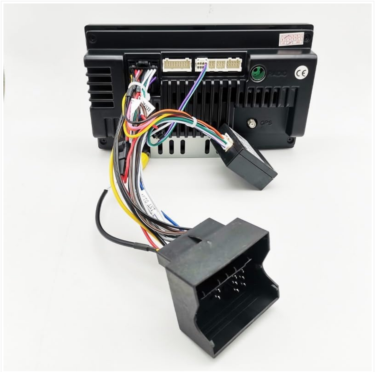
Figure 5.5: The MNBHUYRD wiring harness fully connected to an Android head unit, ready for installation into the vehicle dashboard.
