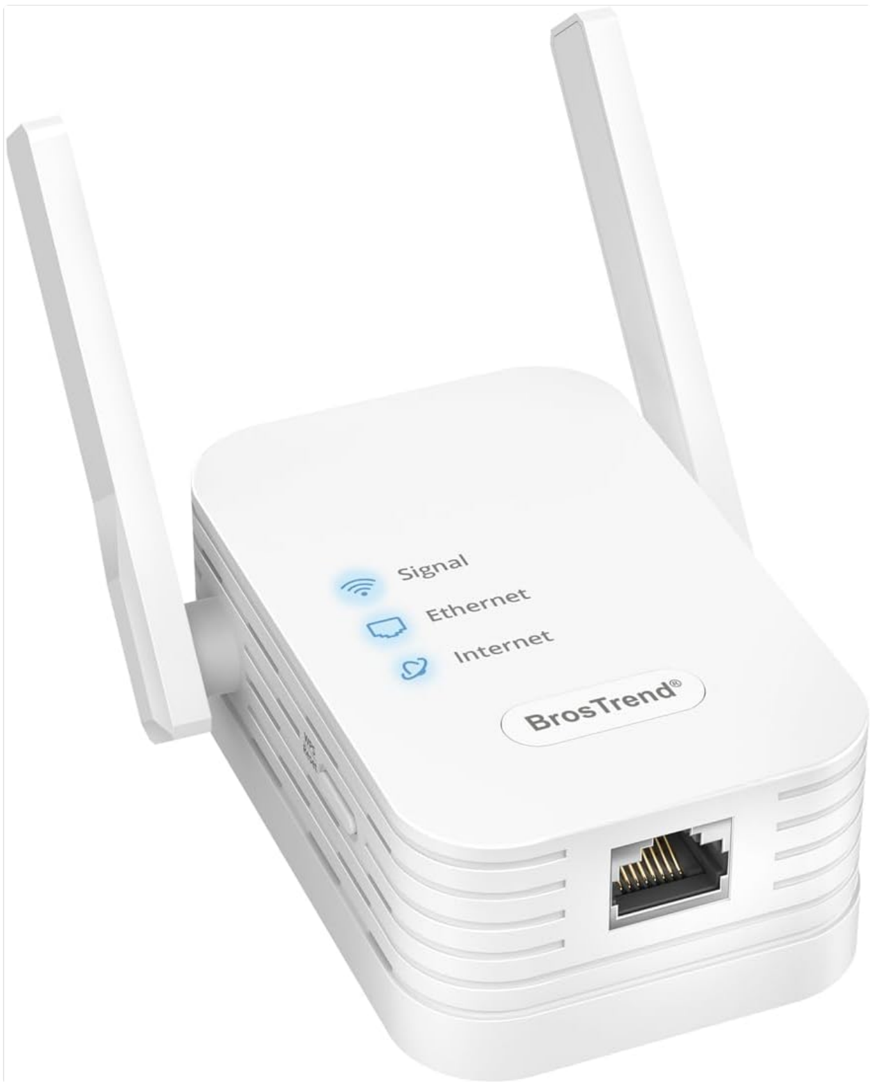
Image 3.1: Front view of the BrosTrend N300 Adapter, showing LED indicators for Signal, Ethernet, and Internet, along with two external antennas.
