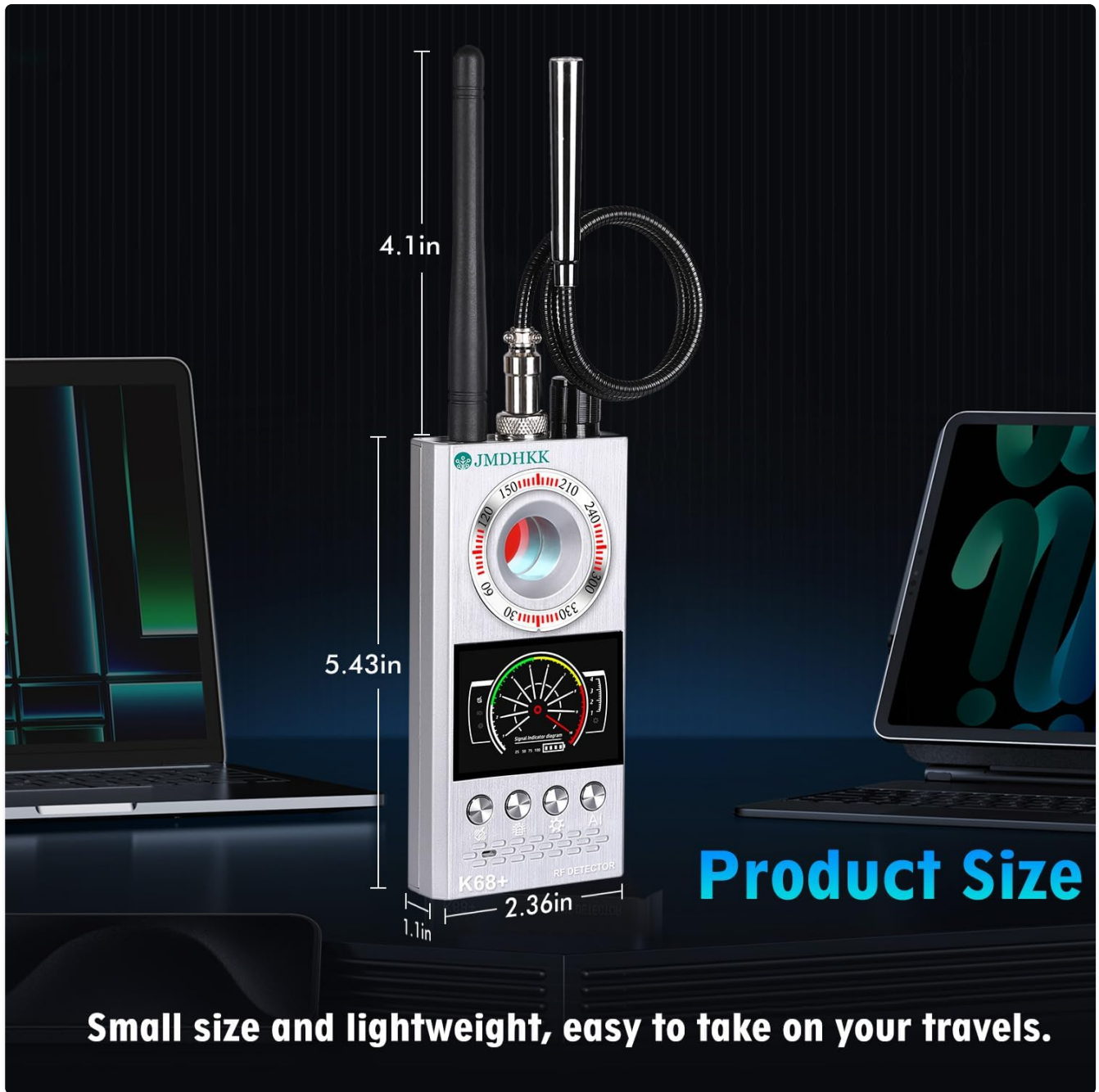
Figure 6: Product dimensions for the JMDHKK K68+ detector.
