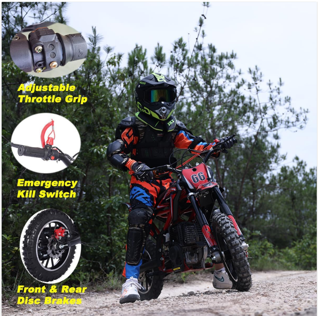
Image 4.1: Key control features including the adjustable throttle grip, emergency kill switch, and front and rear disc brakes.
