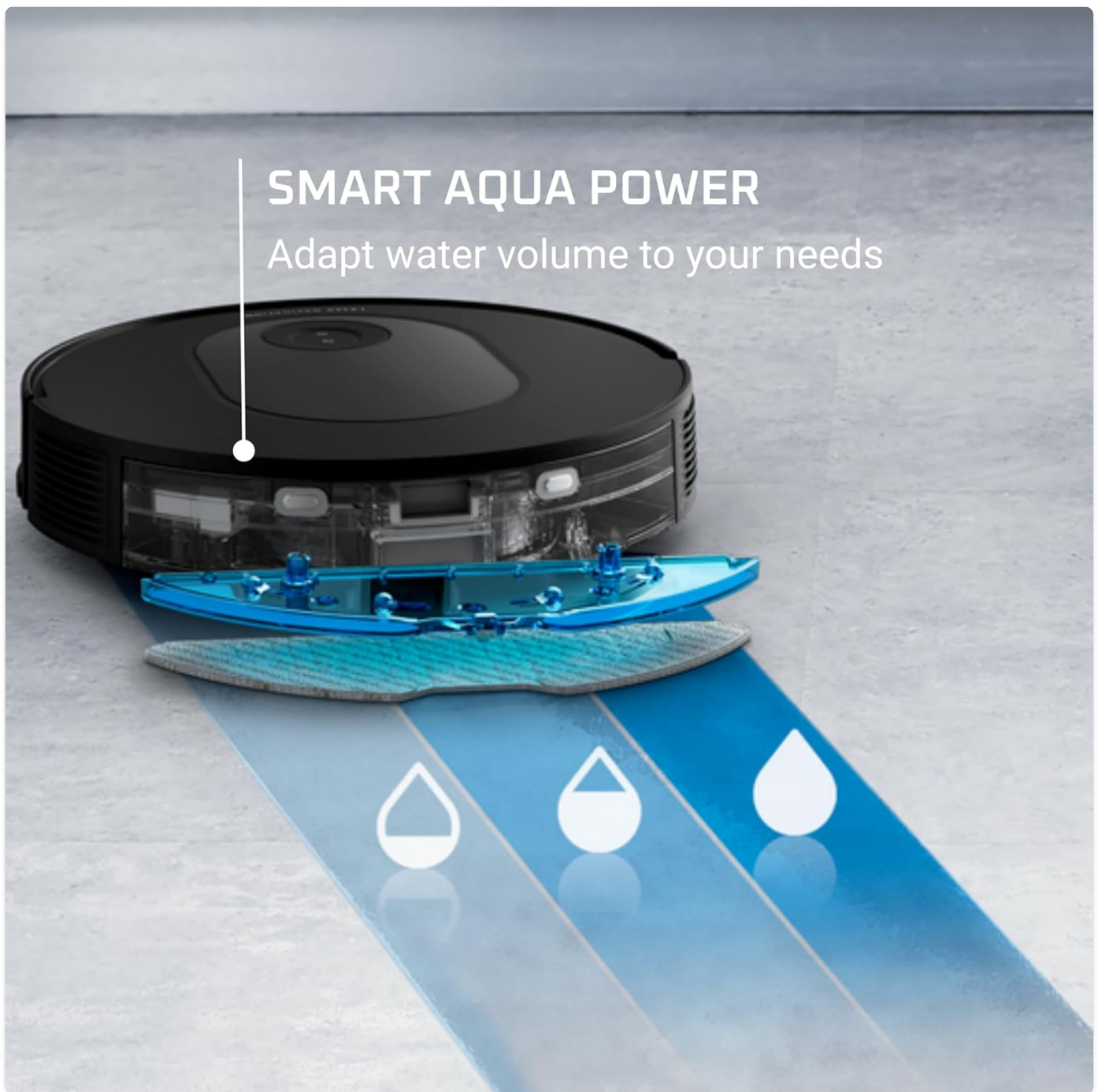
Figure 5: The robot vacuum cleaner on a hard floor, with visual cues of water droplets increasing in size, demonstrating the "Smart Aqua Power" feature that allows users to adapt the water volume for mopping based on their needs.
