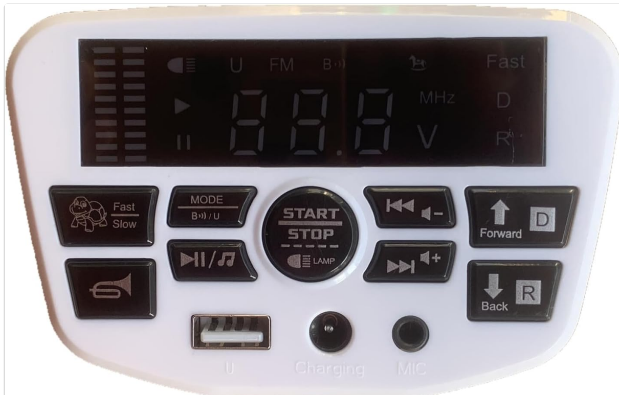
Figure 2.1: Front view of the JR1956G 12V control panel, showing the digital display, various control buttons, and input ports.
