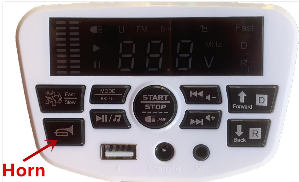
Figure 4.1: Close-up of the JR1956G control panel, highlighting the 'Horn' button and other operational controls.
