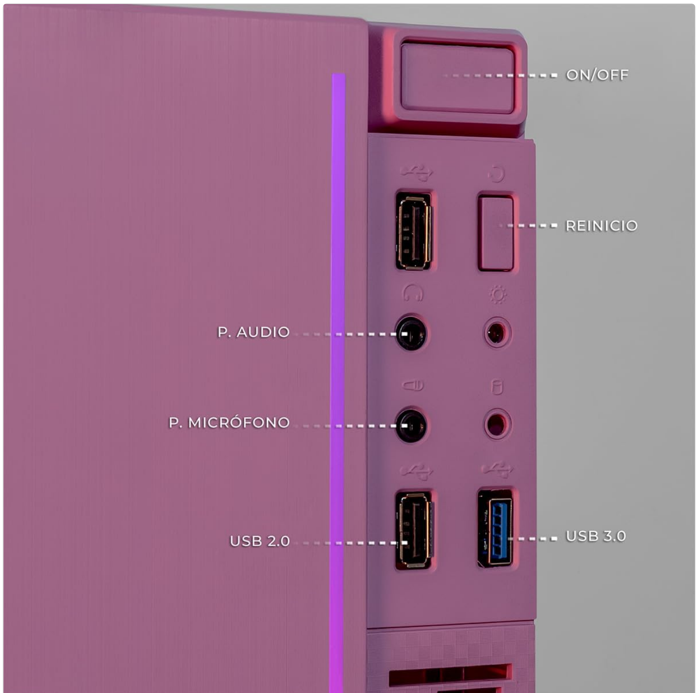
Figure 3: Front panel ports and buttons.
