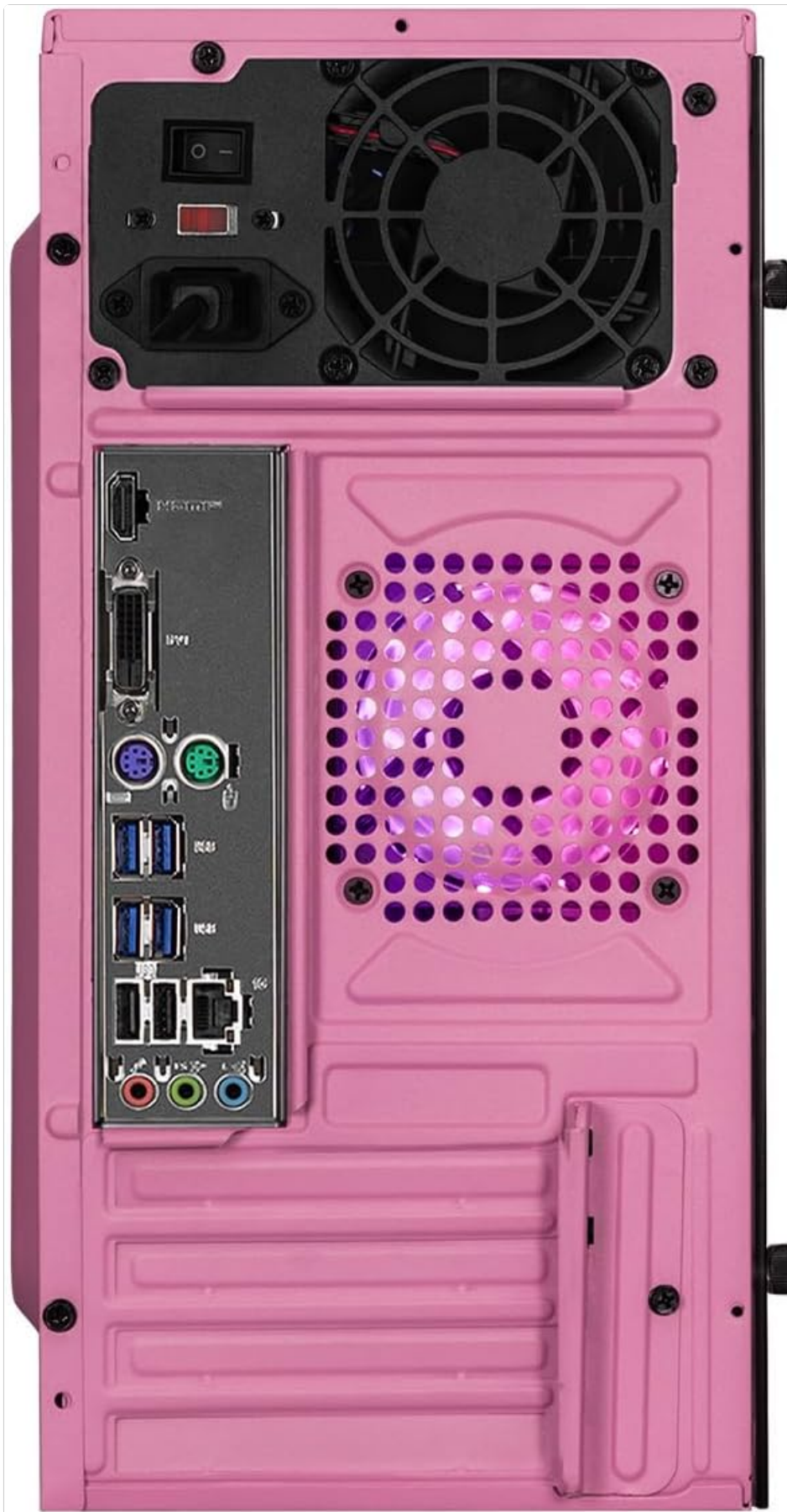
Figure 2: Rear panel connections for peripherals and power.
