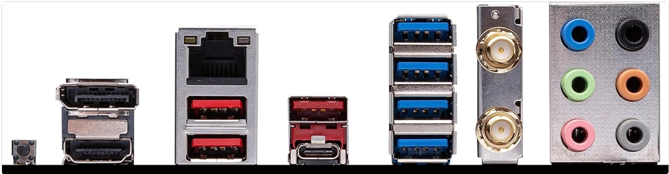
Image: A close-up view of the rear I/O panel, showing various ports including USB, Ethernet, HDMI, DisplayPort, and audio jacks.
