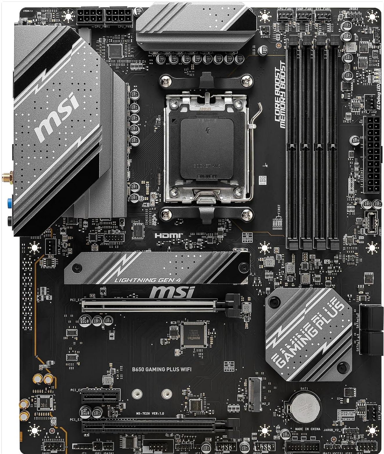
Image: Top-down view of the MSI B650 Gaming Plus WiFi Motherboard, highlighting the CPU socket, RAM slots, and M.2 slots.
