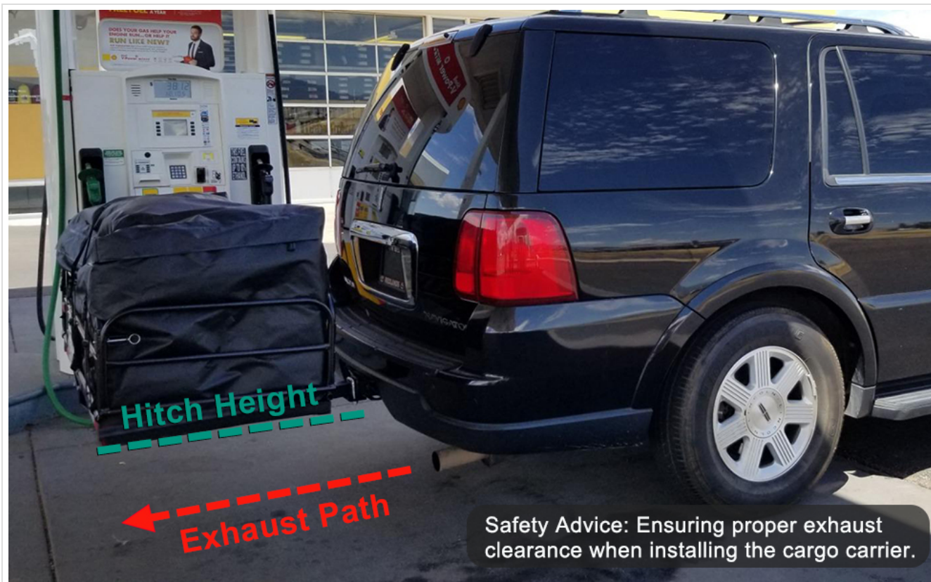
Figure 5: The cargo rack is designed to fit 2-inch receivers and can be folded up when not in use.
