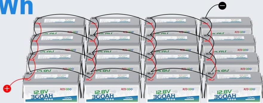
Image 5.1: Examples of battery configurations for expanded power, including parallel and series connections.
