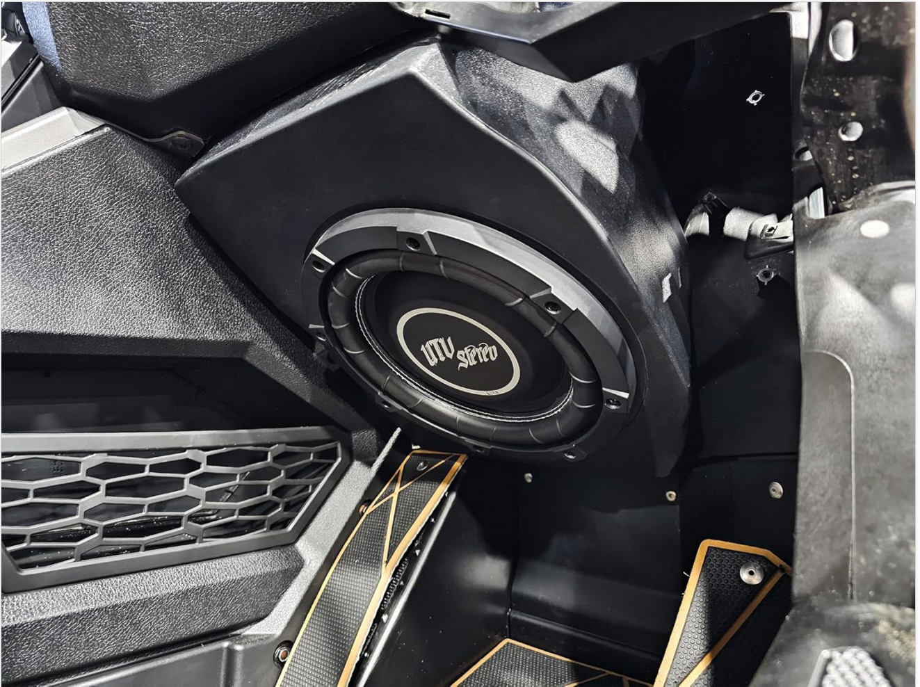
Image: A view of the UTV Stereo RZR Pro Series Vented Dash Subwoofer Enclosure after installation in a Polaris RZR, showcasing its integrated appearance.
