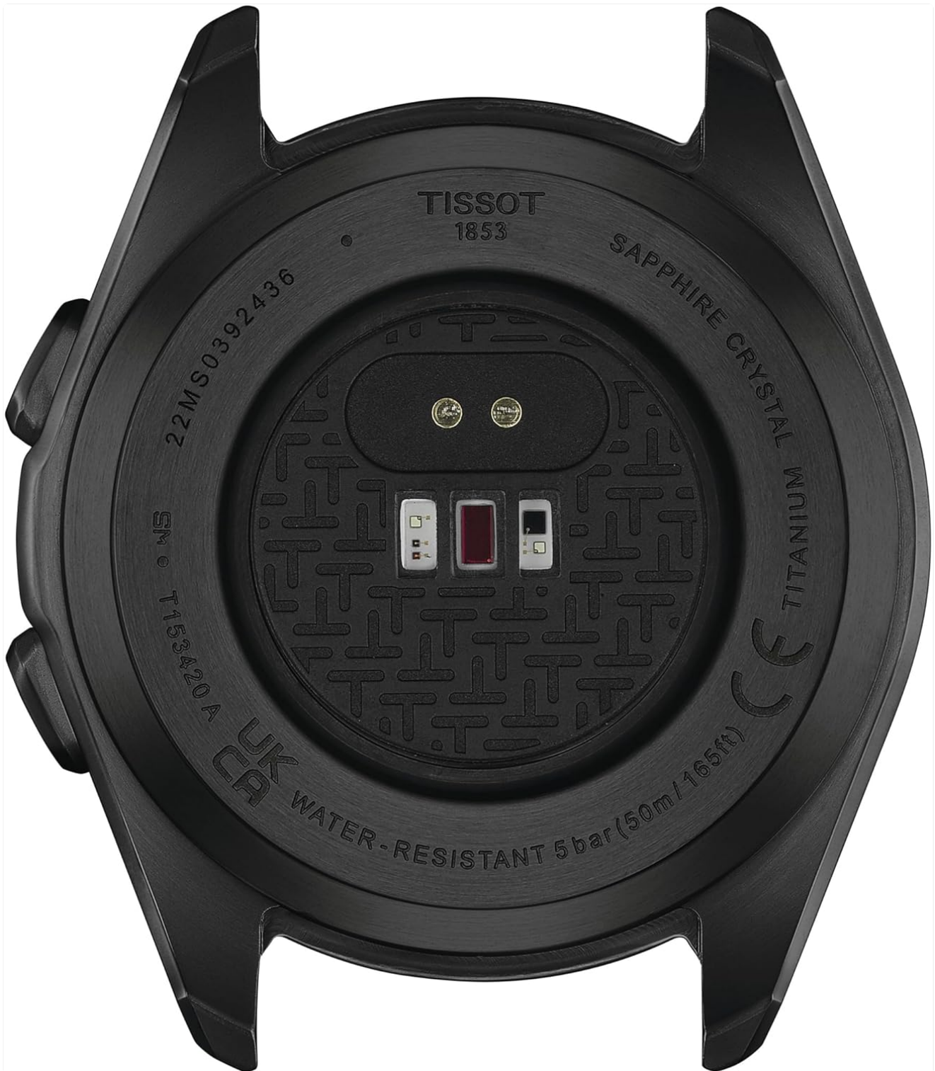
Figure 3.2.1: Rear view of the watch, illustrating the integrated heart rate sensors.
