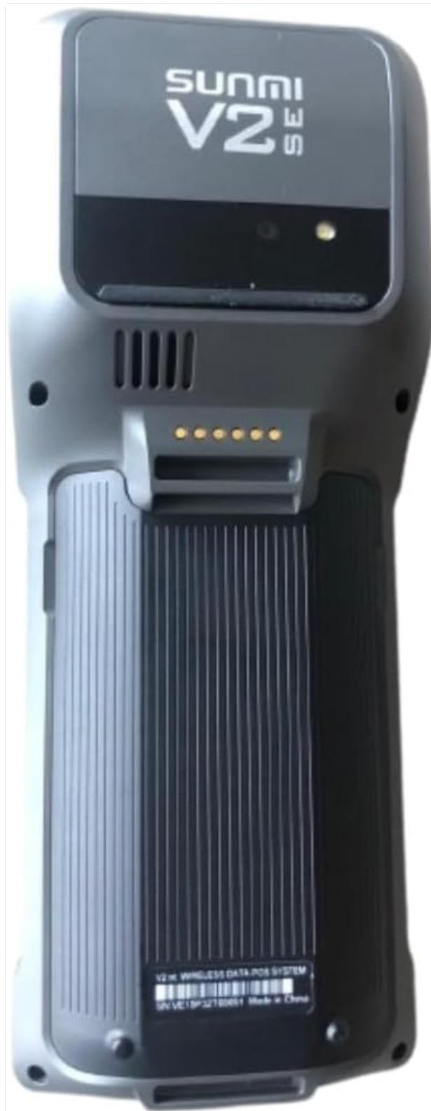
Figure 2.3: Back View. This image illustrates the rear of the device, featuring the thermal printer cover, the 0.3 MP camera, and the charging contact points.
