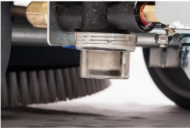
Figure 5: The solution tank, showing the inlet for water and cleaning solution. A measuring cup is used to ensure correct detergent concentration.
