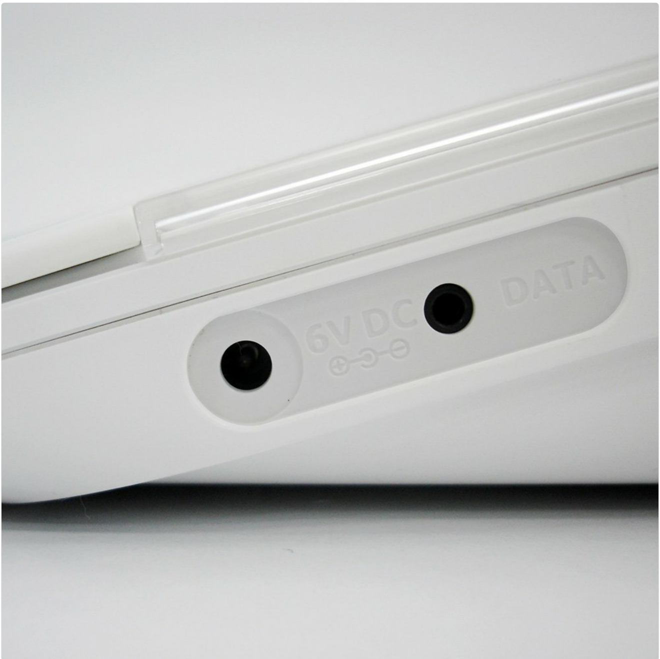
Image: A close-up view of the side of the Rossmax X9 BT PARR PRO monitor, showing the 6V DC power input and DATA ports.
