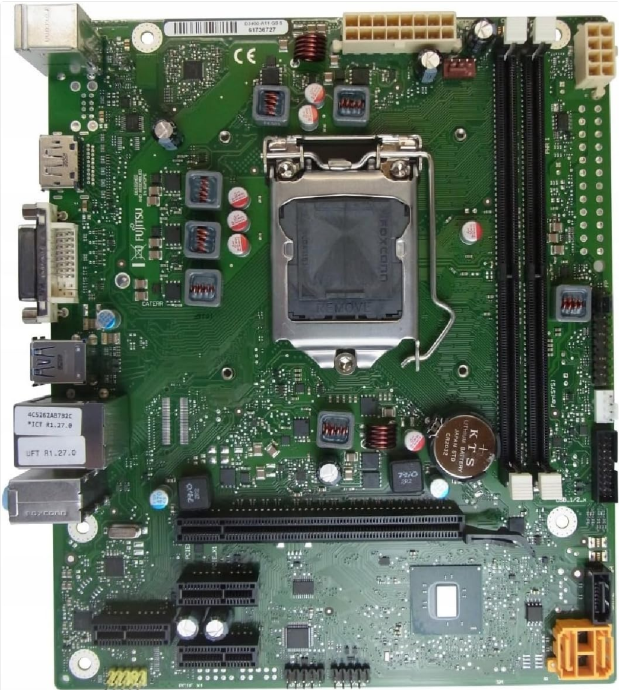
Figure 1: Top-down view of the BQTEC D3400-A11 GS 3 Motherboard, showing the CPU socket, RAM slots, and various connectors.
