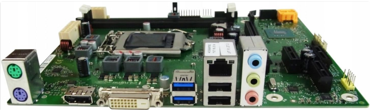
Figure 3: Rear I/O ports of the motherboard, including USB, Ethernet, audio, and video outputs, which should be kept clean and free of obstructions.
