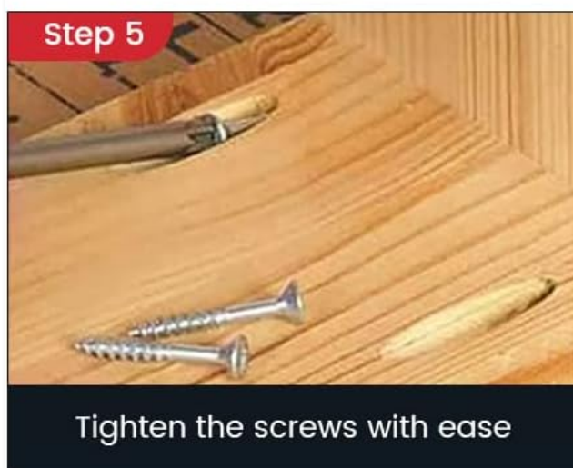
Image 5.1: A six-step visual guide demonstrating the easy operation of the pocket hole jig, from measuring the workpiece to tightening screws and its general use.
