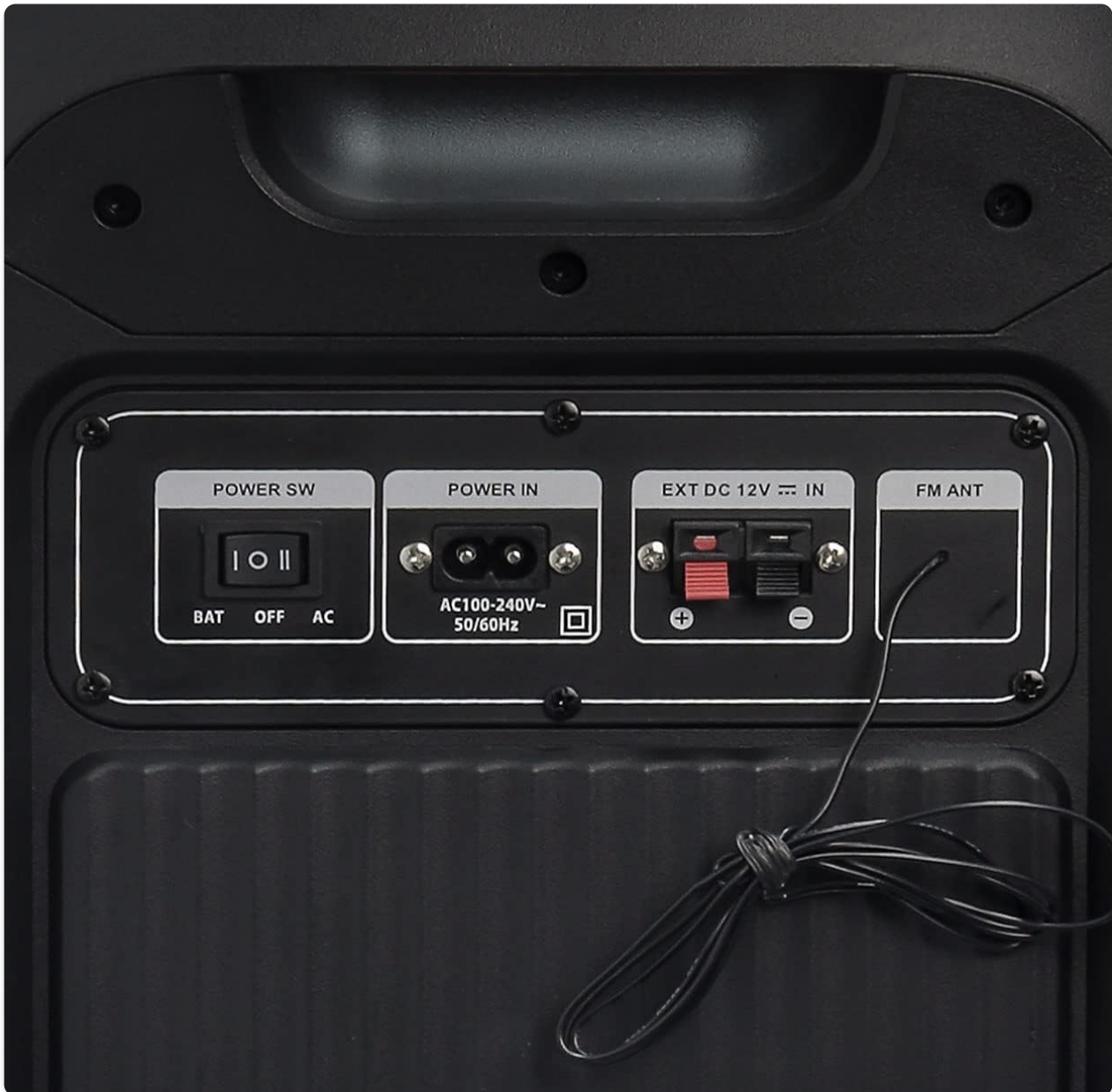
Figure 3: Detailed view of the rear power panel.
