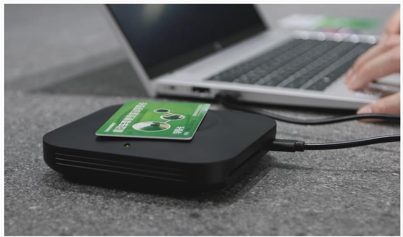
Figure 3.1: The Chainway R1 in operation, connected to a laptop via USB, with an RFID card placed on its surface for reading or writing. This illustrates a typical setup scenario.
