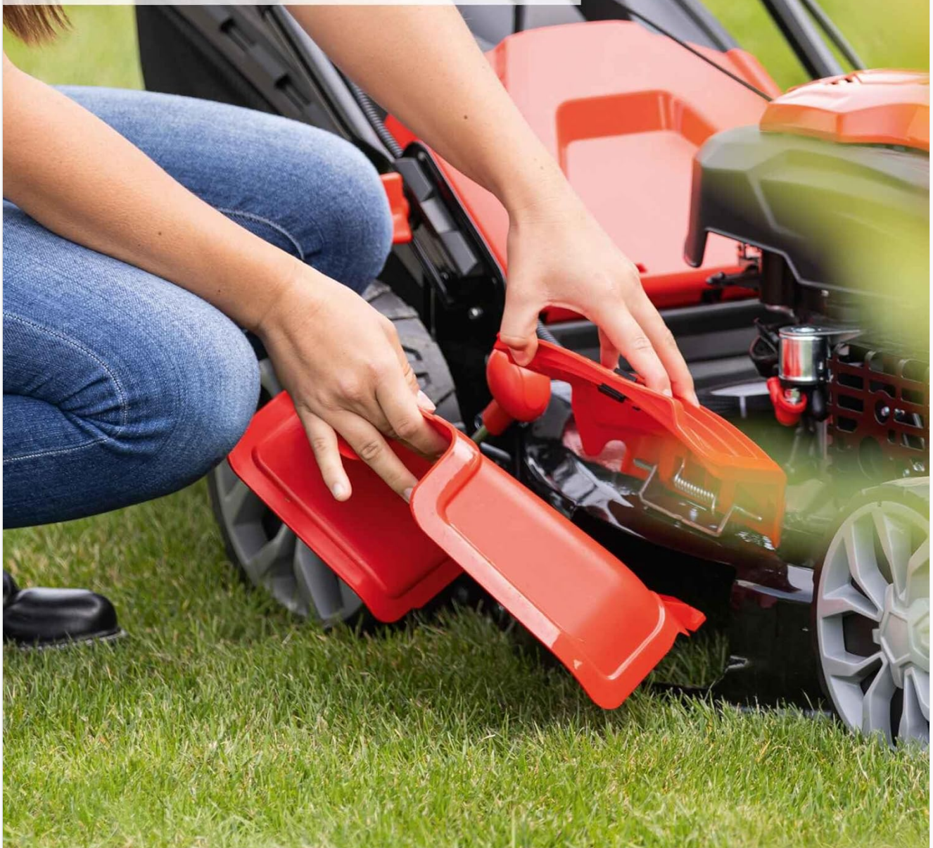
Figure 5.2: The side discharge chute can be easily mounted or dismounted as needed.
