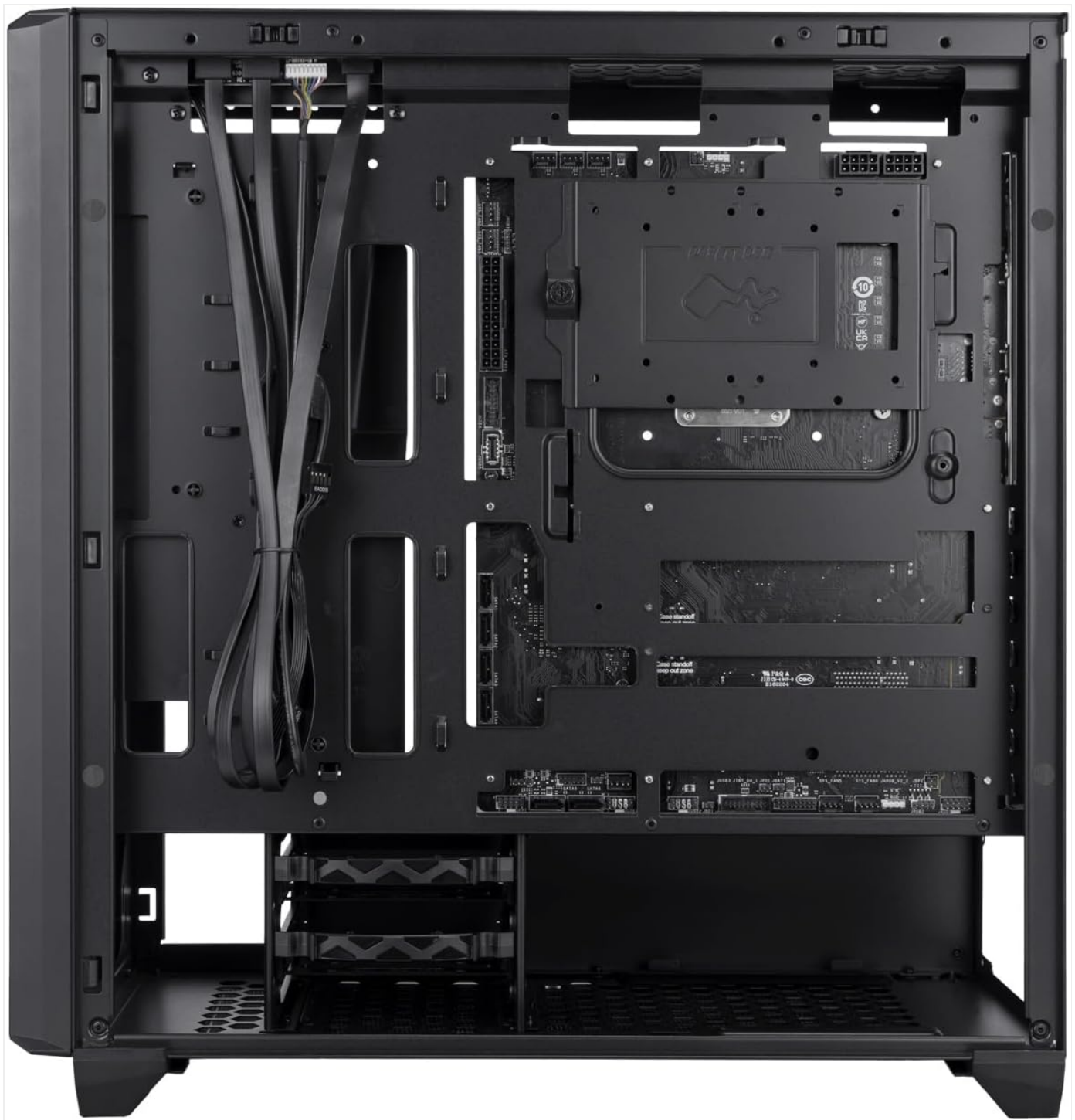
Image: Rear interior view of the IN WIN D5 chassis, highlighting the cable management area and drive bays behind the motherboard tray.
