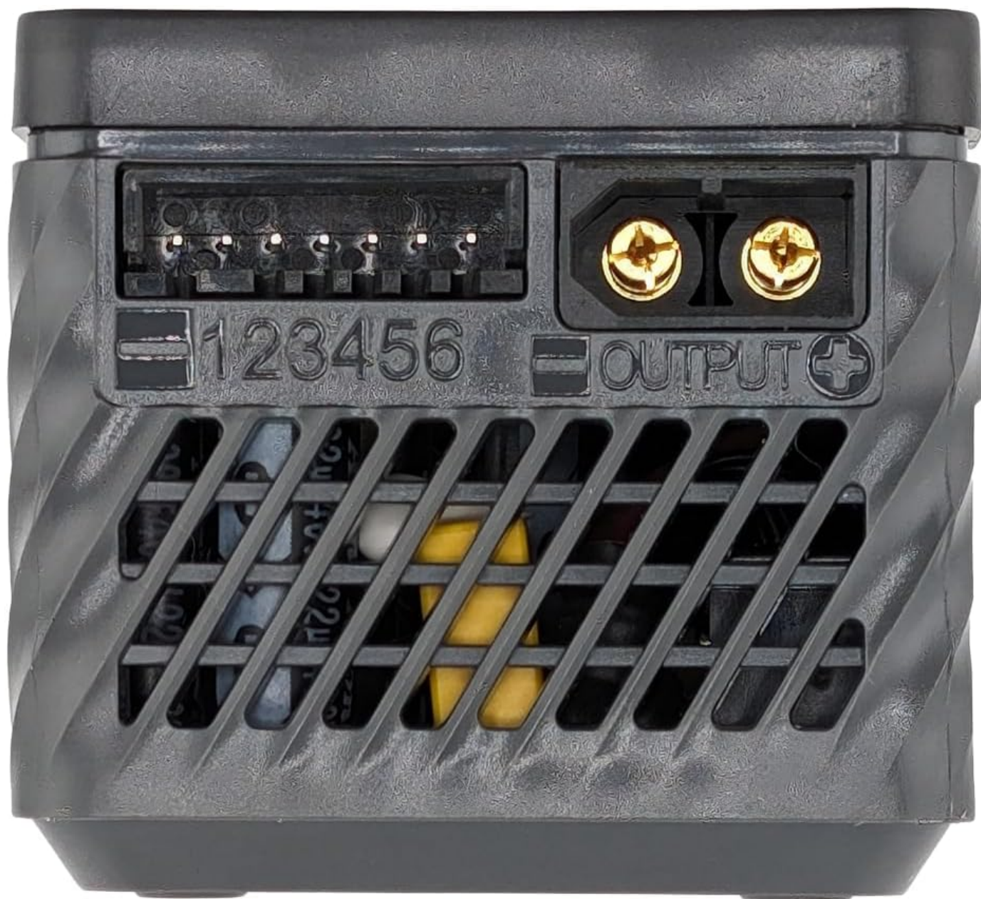
Image: Side view of the charger, showing the main output port and the 1-6S balance port.
