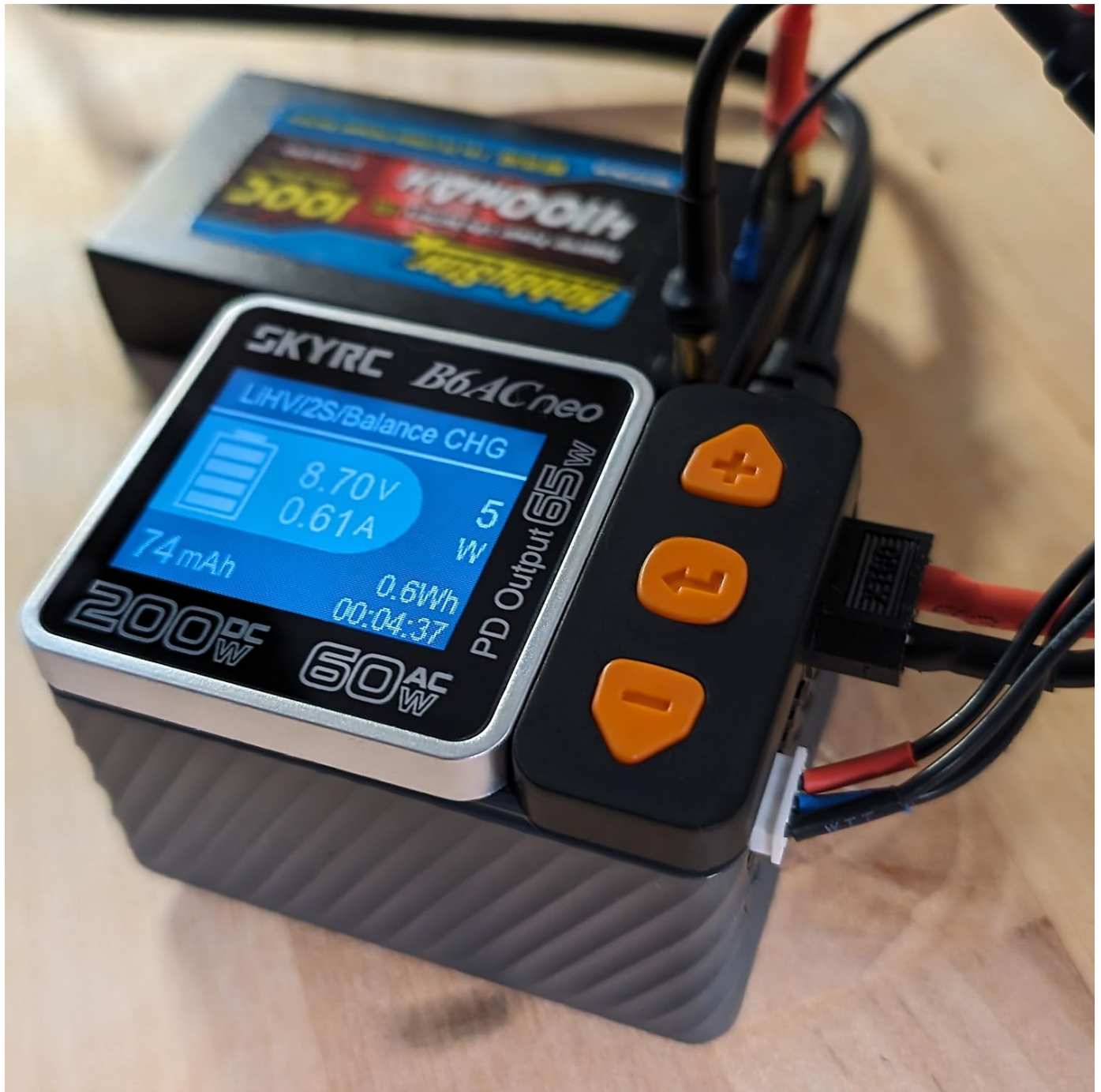
Image: The B6AC Neo in operation, displaying charging voltage, current, and capacity for a LiHV battery.
