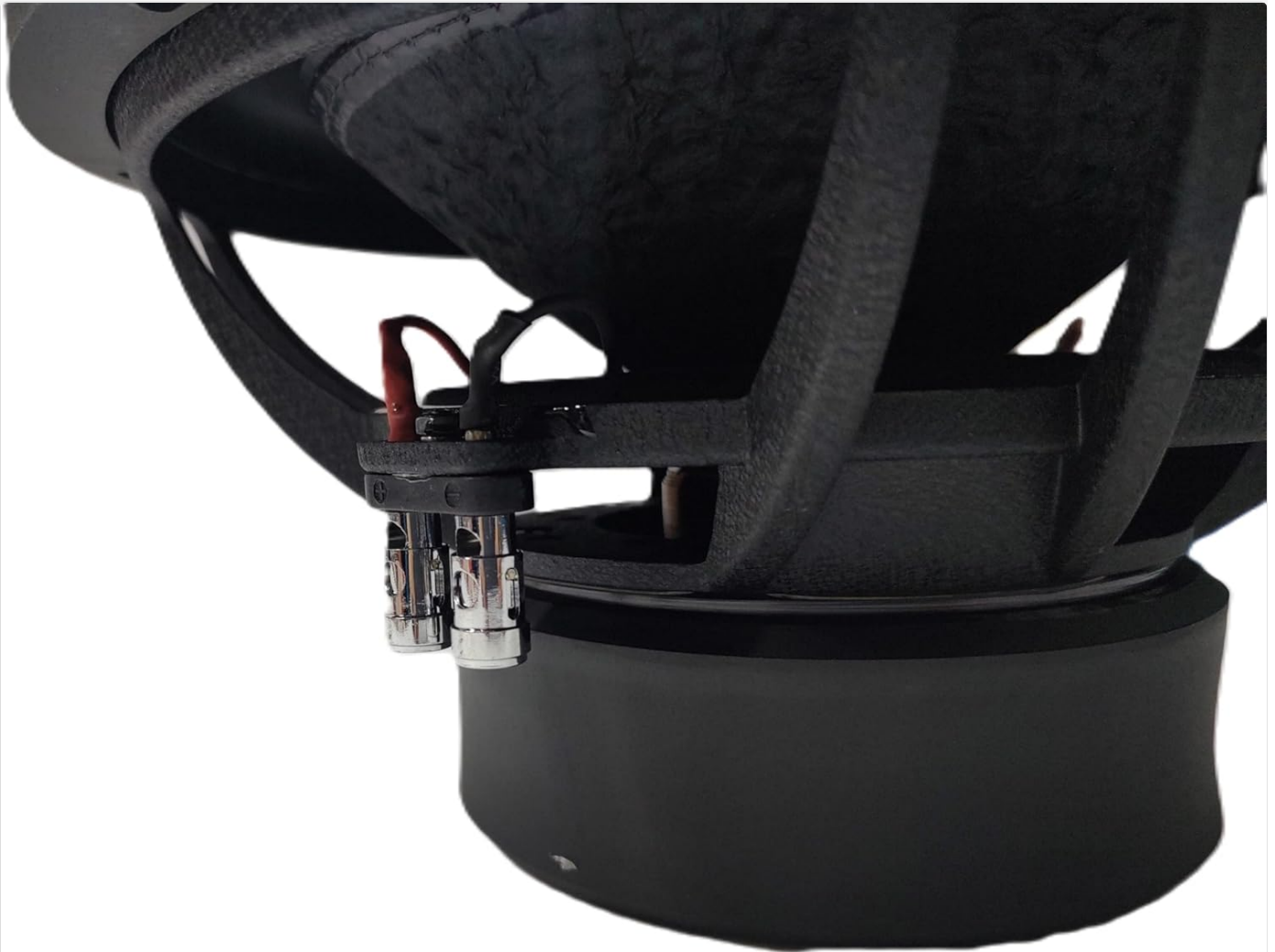
Figure 5.1: Subwoofer Terminals for Wiring
