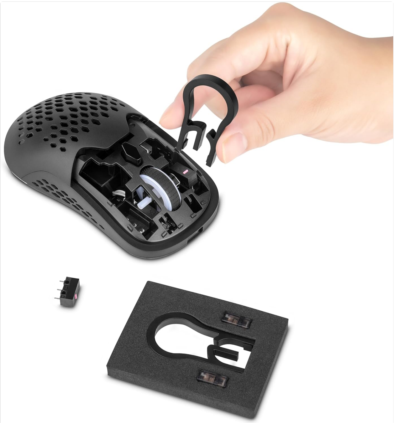
Figure 3.3: Demonstration of removing a Kailh GM8.0 switch, highlighting the swappable switch design.
