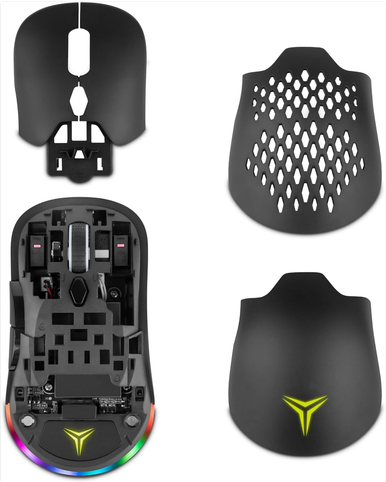
Figure 3.2: Exploded view illustrating the two interchangeable covers and the mouse's internal structure.
