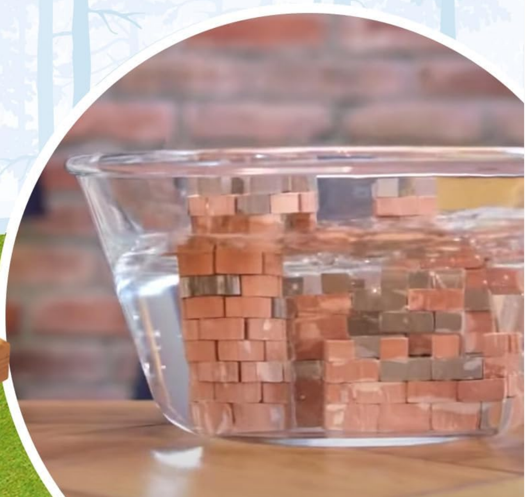
Image: The process of dissolving the glue in water to enable brick reusability.
