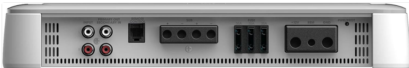
Figure 2: Rear view of the JBL MA1000 amplifier, illustrating the power, ground, remote, input (RCA), and subwoofer output terminals, along with the fuse holders and remote control port.
