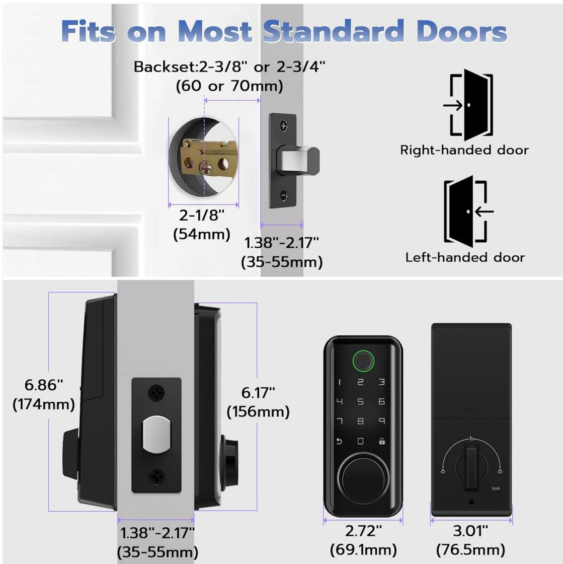
This diagram illustrates the required door dimensions for installing the Eseesmart Smart Door Lock, specifying the backset (60mm or 70mm), door thickness (35-55mm), and bore hole diameter (54mm). It also shows compatibility with both right-handed and left-handed doors.
