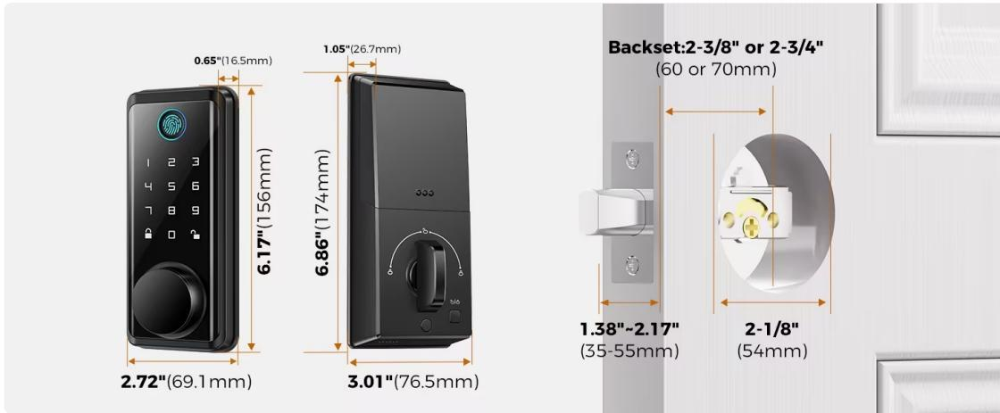
This image presents the detailed dimensions of the Eseesmart Smart Door Lock's exterior and interior units, along with the deadbolt mechanism, including measurements for length, width, and height in both inches and millimeters, and backset specifications.
