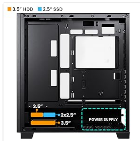
Figure 4.4: Diagram illustrating the locations for 3.5" HDDs and 2.5" SSDs within the chassis.
