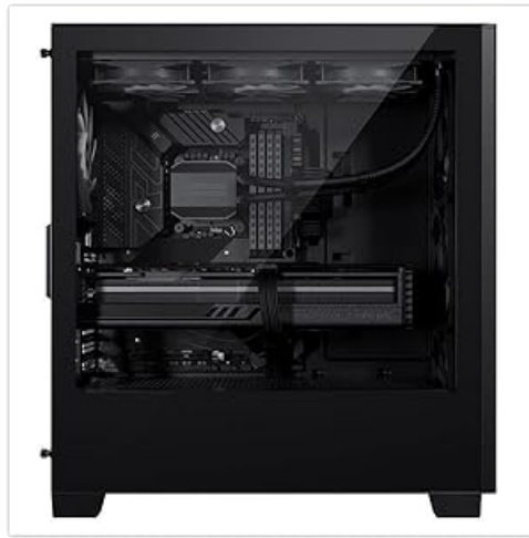
Figure 4.3: Interior view of the Phanteks XT Pro with a motherboard, CPU cooler, and graphics card installed.
