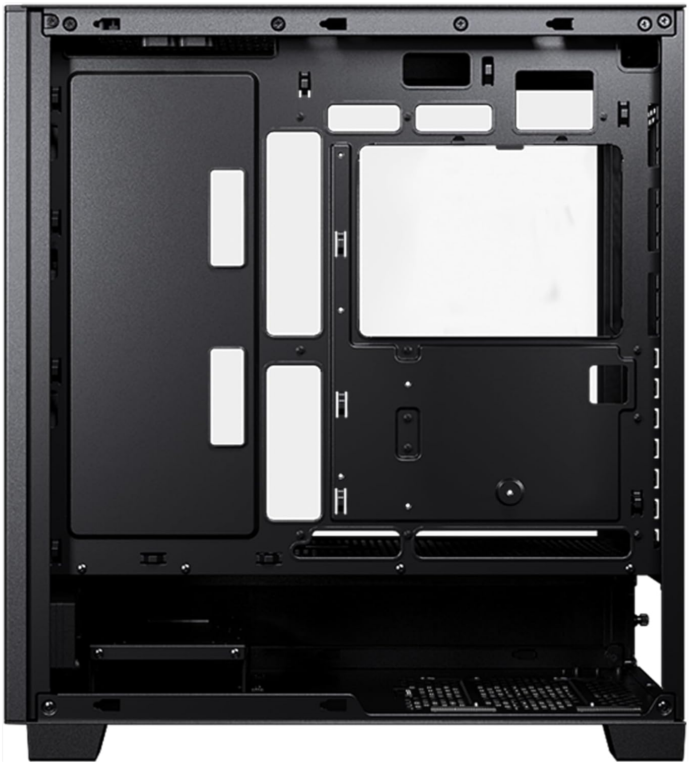
Figure 4.2: Rear interior view of the chassis, showing cable management routes and drive mounting locations.
