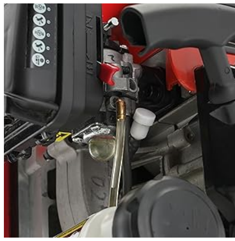
Figure 5.1: Location of the primer bulb for engine starting.
