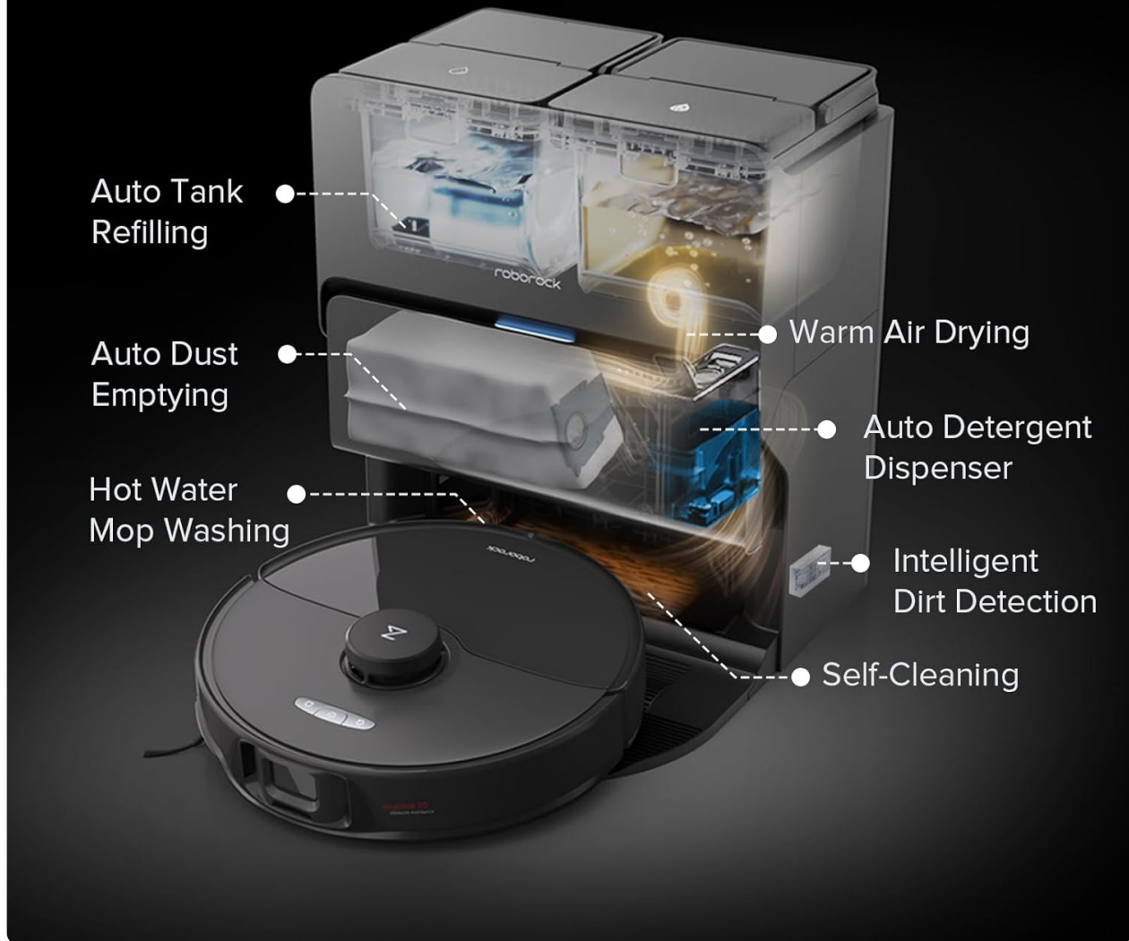
Figure 2: Key features of the All-in-One RockDock Ultra, including automatic tank refilling, dust emptying, hot water mop washing, and intelligent dirt detection.
