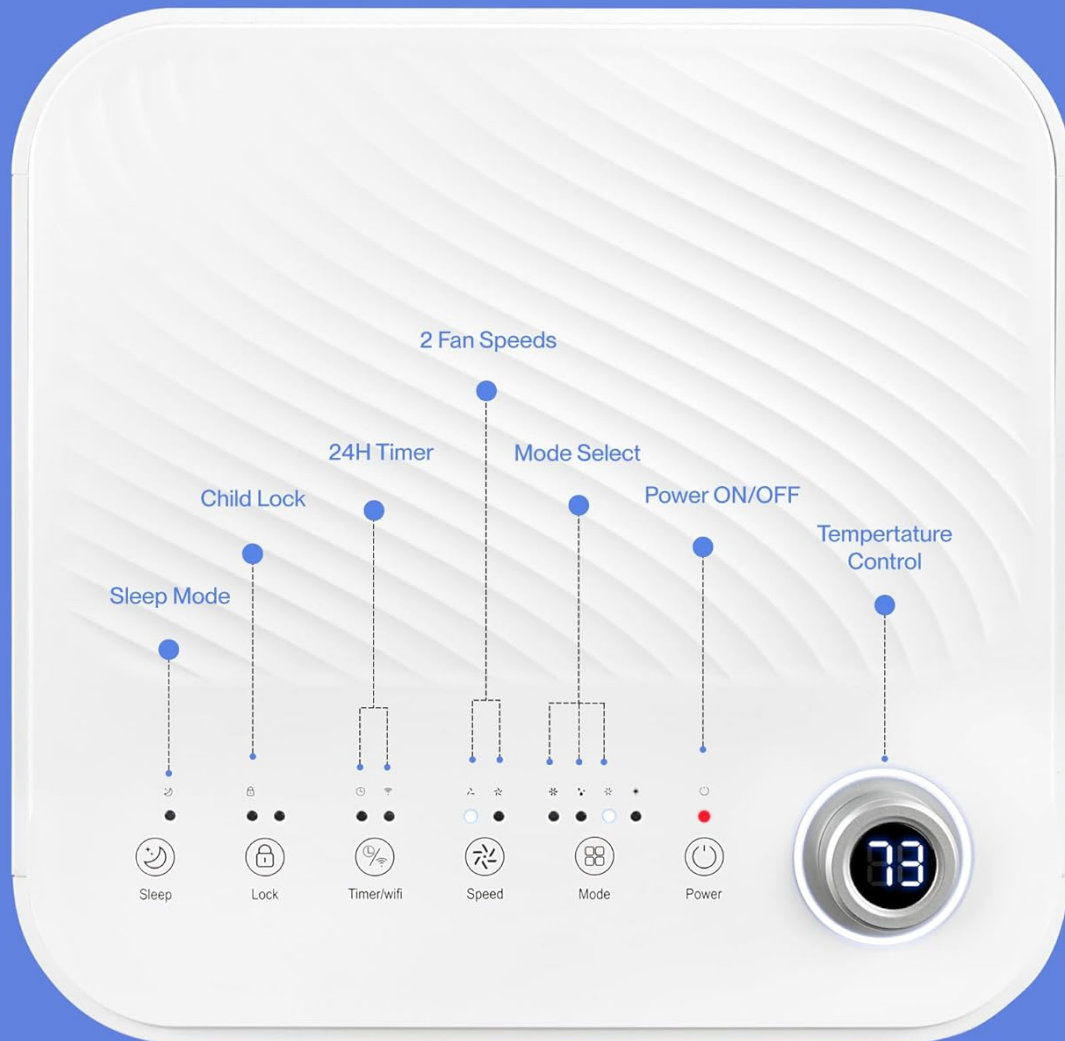
Figure 4.1: The intuitive top-mounted control panel with LED display for easy operation.
