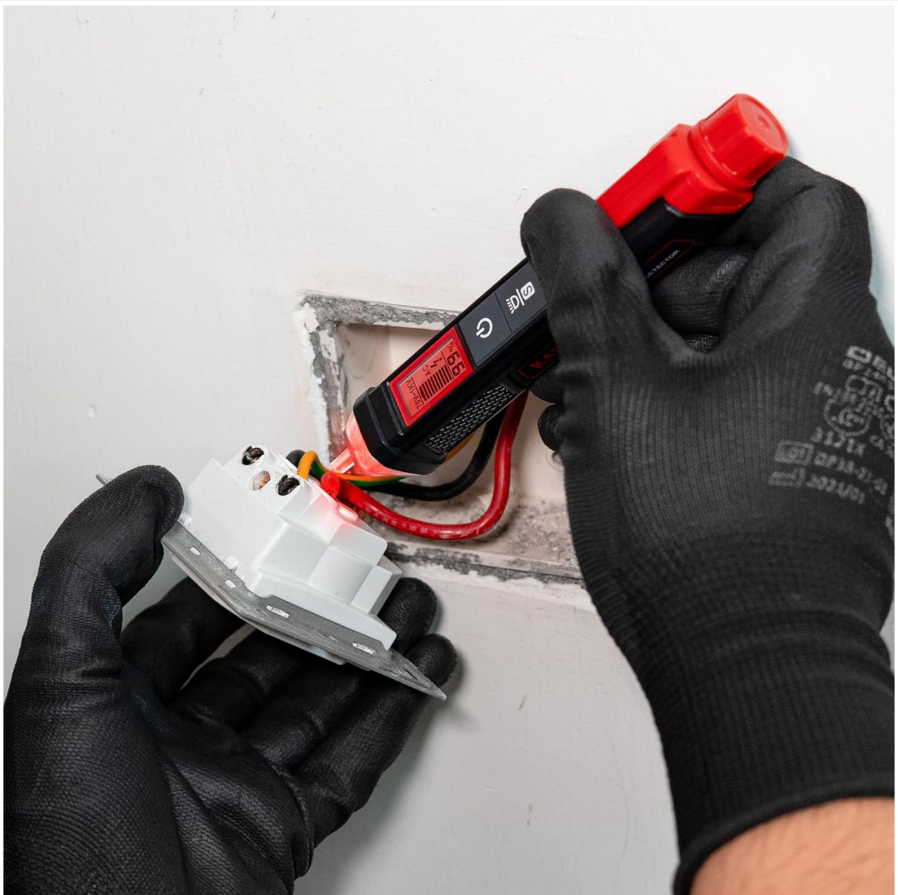
Figure 5.5: NCV Tester in use on an electrical outlet. The image shows the HT100s NCV tester's tip near the wiring of an exposed electrical outlet, with the tip glowing red, indicating the presence of voltage. This demonstrates the non-contact voltage detection feature.
