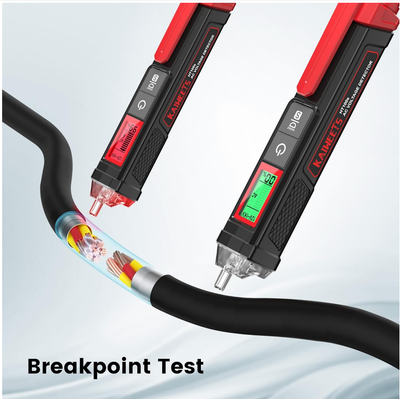
Figure 5.6: Breakpoint Test using the HT100s NCV Tester. The image shows two HT100s testers, one indicating voltage on a transparent cable (showing internal wires) and another further along the cable not indicating voltage, demonstrating how to locate a break in a wire.
