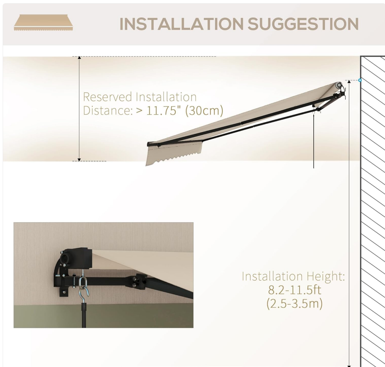
Image 3.1: Recommended installation height (8.2-11.5ft) and reserved distance (>11.75") for the awning.
