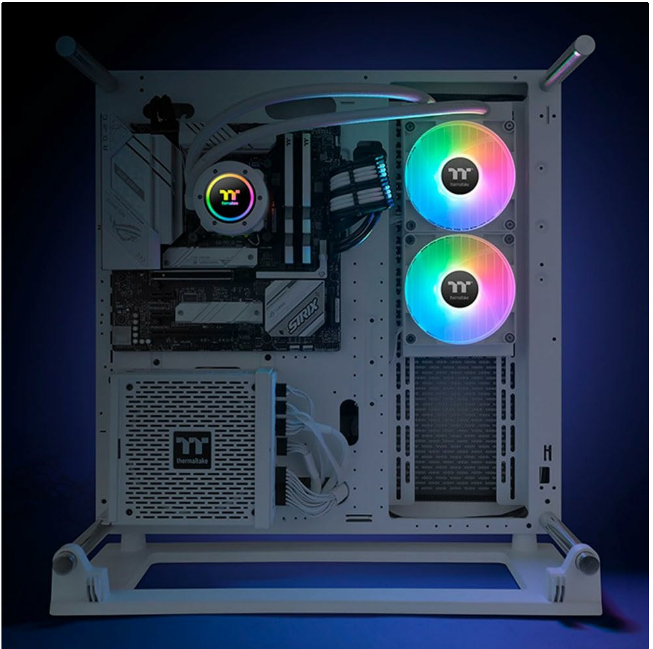
Figure 5: The TH240 V2 ARGB cooler installed in a white PC build, showing the radiator mounted at the top and the illuminated pump and fans.
