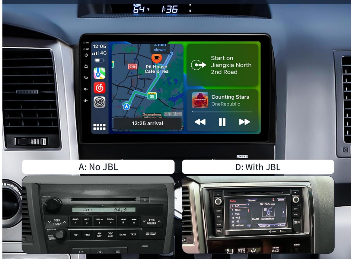
Figure 1.1: Compatibility overview, illustrating the difference between factory radios without JBL (Model A) and with JBL (Model D) to ensure correct harness selection.
