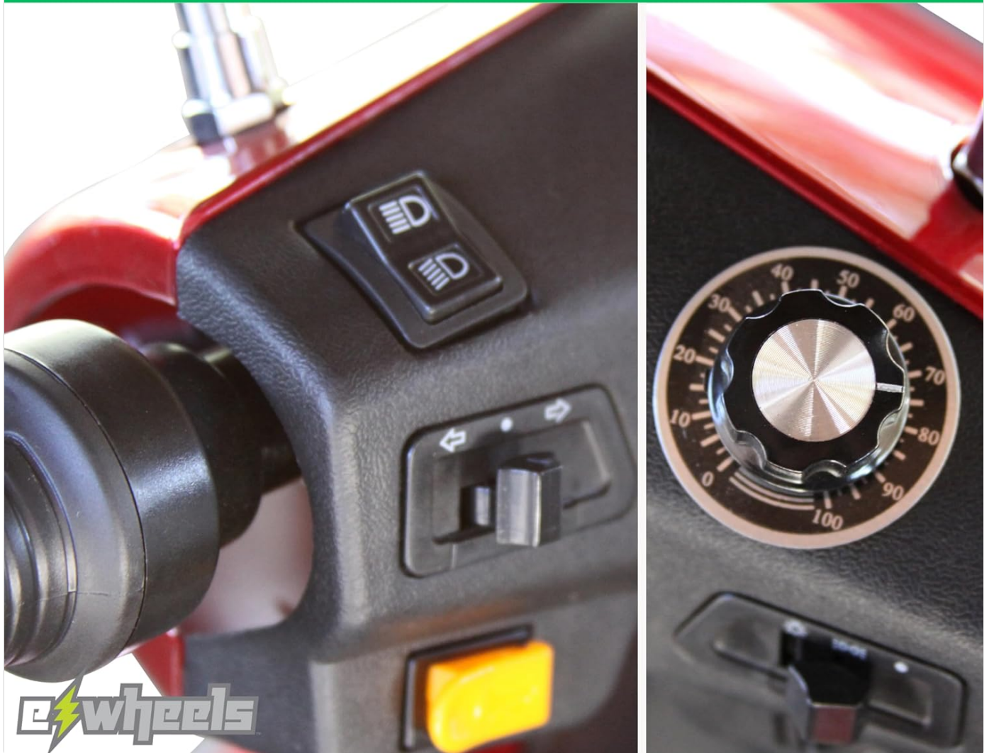
Image: A detailed view of the EW-36 scooter's controls, including the headlight switch, turn signal switch, and a dial for speed adjustment, labeled "Easy to Operate".
