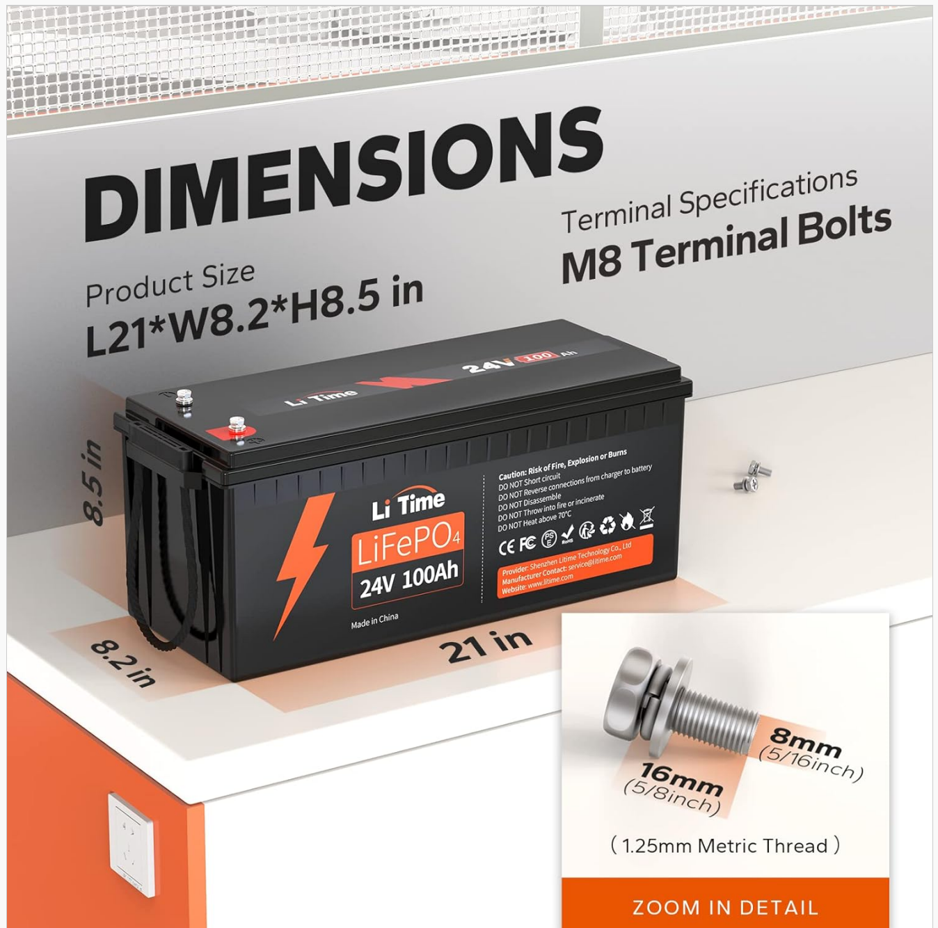
Figure 2: The battery dimensions are 21 inches (L) x 8.2 inches (W) x 8.5 inches (H). The M8 terminal bolts have a diameter of 8mm and a length of 16mm with a 1.25mm metric thread.
