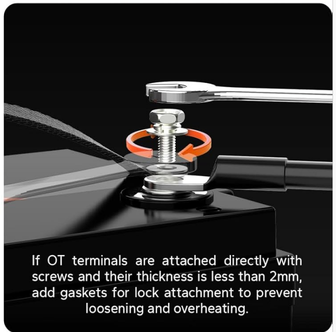
Figure 3: Important usage guidelines: Do not use for golf carts or engine starting. For thin OT terminals, add gaskets to ensure secure connections and prevent overheating.
