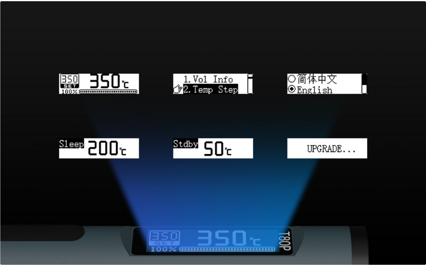
Image: Various OLED display screens, including temperature display, volume info, temp step, sleep mode, standby mode, upgrade option, and language selection (Simplified Chinese and English).
