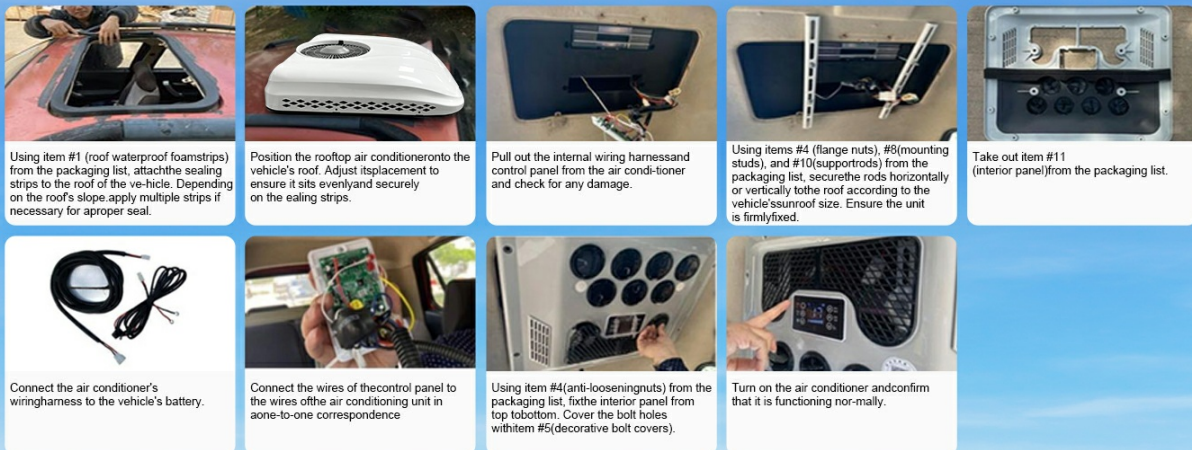
Image 5.1: A visual quick installation guide showing 8 steps. These steps include: 1. Applying waterproof foam strips to the roof opening. 2. Positioning the rooftop AC unit. 3. Pulling out the internal wiring harness and control panel. 4. Securing the rods horizontally or vertically. 5. Taking out the interior panel. 6. Connecting the AC unit's wiring harness to the vehicle's battery. 7. Connecting the wires of the control panel to the AC unit and installing the interior panel. 8. Turning on the AC unit to confirm normal function.
