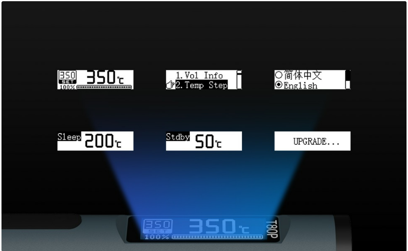
Image: Examples of information displayed on the OLED screen, including temperature, settings, and status.
