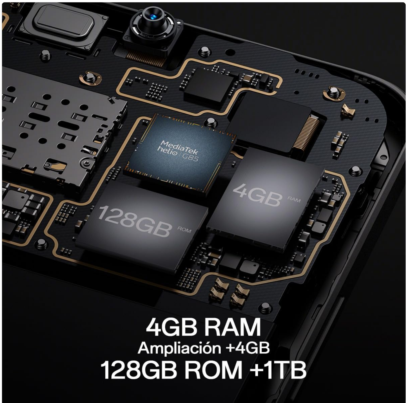
Figure 4.3: Internal view of the OPPO A18 showcasing the MediaTek Helio G85 processor, 4GB of RAM (expandable), and 128GB of internal storage (ROM).
